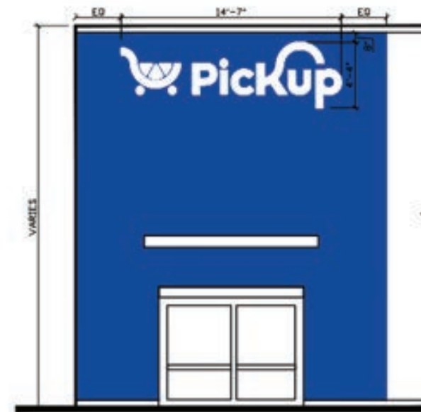
TYPICAL PAINTED AREA: PICKUP FRONT ENTRY DOOR NEAR CORNER - CENTERED HORIZONTALLY OVER CANOPY/DOOR AND OR AT LEAST 1'-6" FROM CORNER OF BUILDING. CREATE PAINT FINISH BREAK ON OPPOSITE SIDE EQUAL DISTANCE FROM EDGE OF SIGN LEFT & RIGHT.
