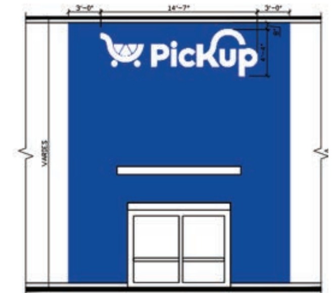
TYPICAL PAINTED AREA: PICKUP FRONT ENTRY DOOR ON BLANK FACADE - CENTERED HORIZONTALLY OVER CANOPY/DOOR. INSTALLED 8-12" FROM BOTTOM OF CORNICE/COPING - or - CENTERED VERTICALLY BETWEEN CANOPY OR DOOR AND CORNICE/COPING. CREATE PAINT FINISH BREAKS 3' MINIMUM FROM EDGE OF SIGNAGE.
